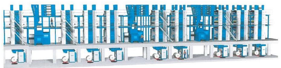
9 printing towers / 3 Folders / 9 Reelstands - Large diameter reel (1500 mm) / 2 AGV
